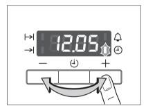
After approx. 5 seconds, the flashing stops and the clock displays the time set.
